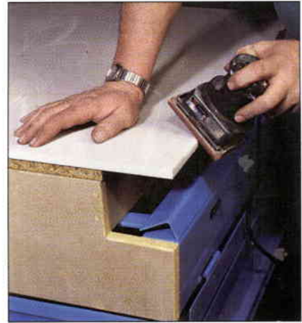
Chip deflector in down position for sanding edges
