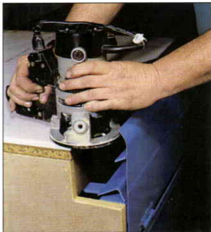
Chip deflector in up position for use with router
