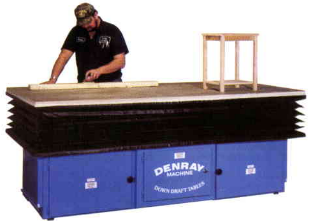
Top in up position to sand flat goods
