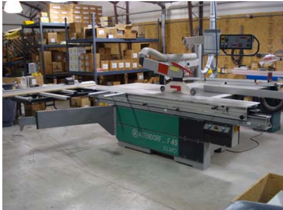
Altendorf F-45 3200 ELMO 3 Sliding Table Panel Saw
