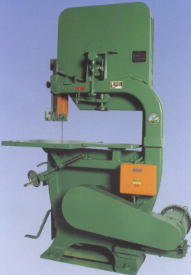
Rear view of 32" Heavy-Duty Bandsaw showing Belt Drive configuration.
