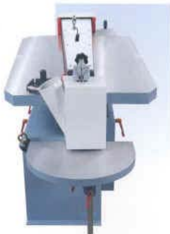
Double Table for Powerful Sanding Corner Sanding Table for Curved Sanding
