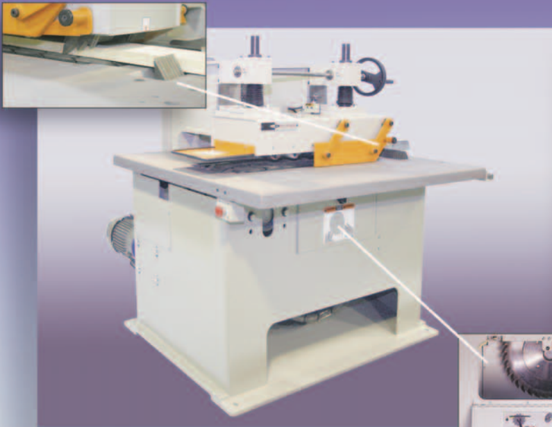
The front view illustrates access into the electrically interlocked saw pit area, the dual anti-kickback finger system and the pivoting pressure beam side guard.
