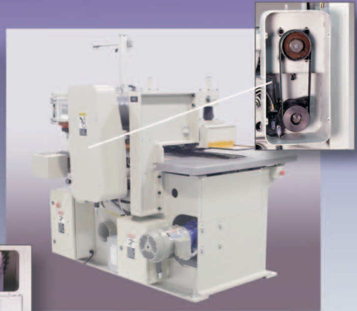
The machine's back side is shown with the arbor drive housing cover removed to depict the automatic arbor brake.
