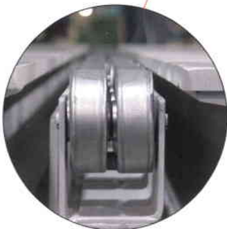
5. Retractable rollers in lower platen to assist in material handling
