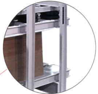
3. Pre-set 28" (711 mm) opening to accommodate a full bunk of board for each pressing cycle
