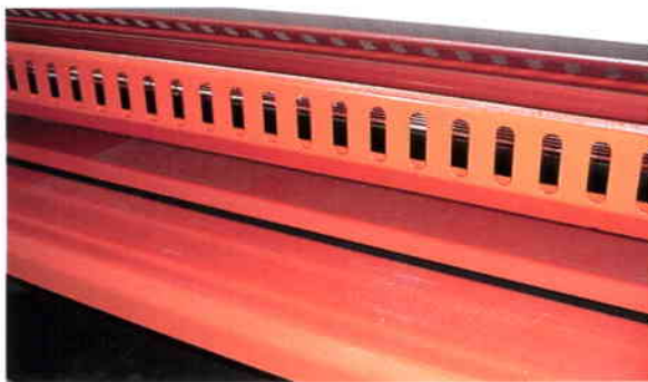
Pivoting infeed table guard and infeed barrier guard
