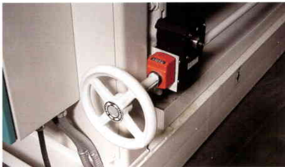
Single Handwheel Doctor Roll Adjustment
