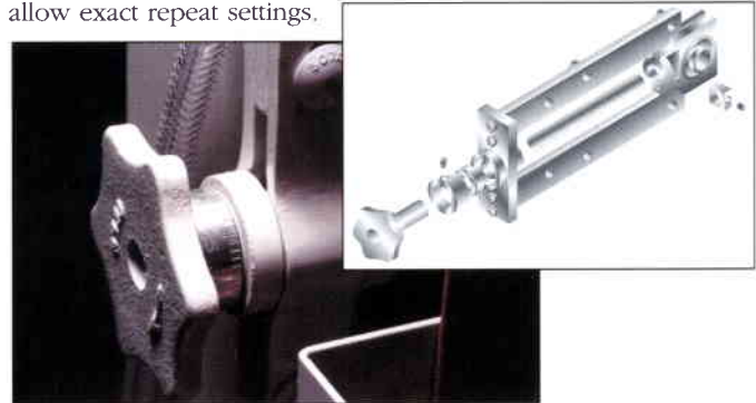
Micrometer scale doctor roll adjustment
