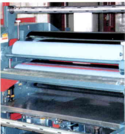
Optional outfeed resilient covered combining rolls ensure conformance to uneven boards.
