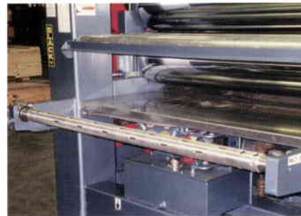
Air shafts are offered as an option to dramatically improve paper changeover times to improve productivity.
