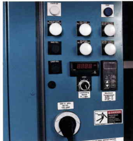
Numerical controls provide operator with highly accurate method of maintaining oil temperature and line speed.
